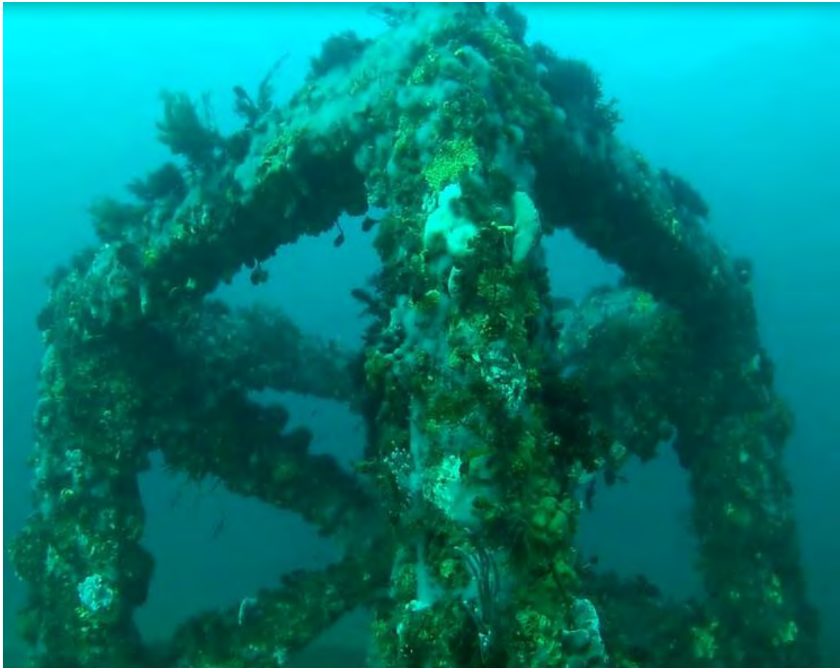
Figure 1: A previously bare surfaced concrete module from the South West Artificial Reef Trial in WA.
