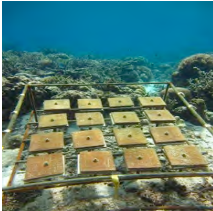
Fig. 2.1. Settlement tiles placed on raised racks (from Fig. 9 in Bremen (2014)).
