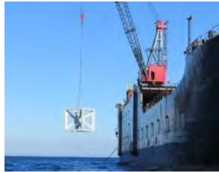
Concrete fish boxes made by Hae Joo. Boxes are 4 m 3 and weigh 14.4 T.
