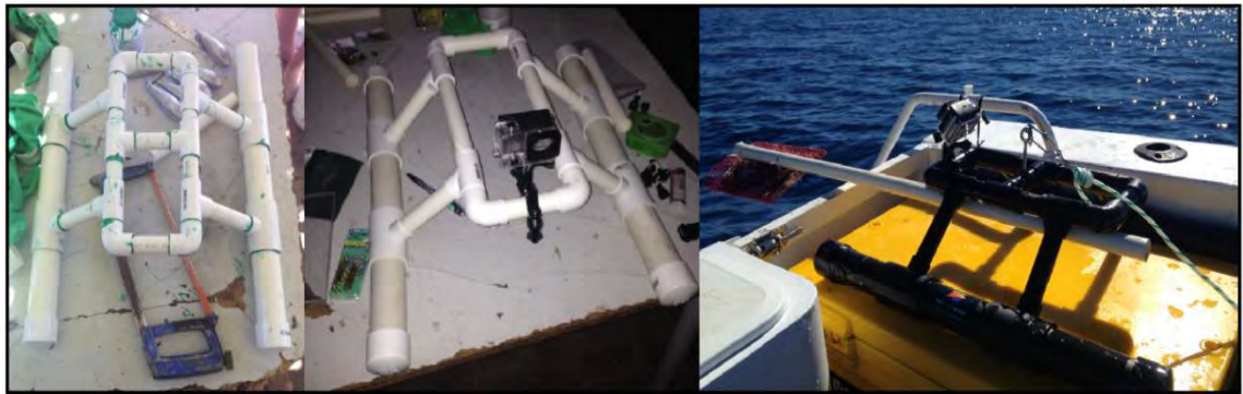
Fig. 4.1: Construction of the custom made BRUV. From right to left: Cementing pipe fixtures with weights already inside the legs (skids), the finished BRUV frame trialling with camera position, and final product about to be deployed on the artificial reef.
