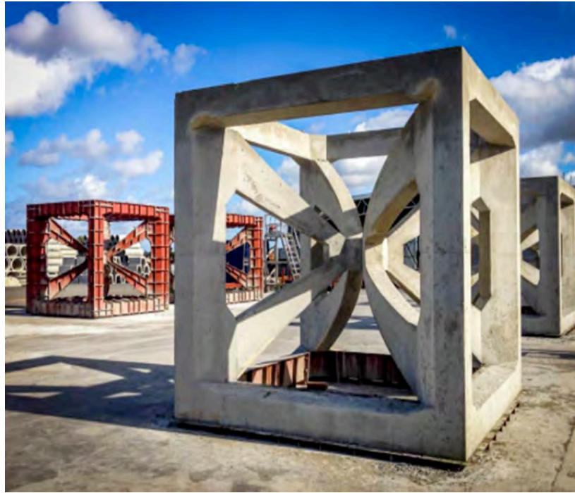
Fig. 3.2. An image of a 'Fish Box' unit, deployed as part of the South West Artificial Reefs Trial (Haejoo, 2016).
