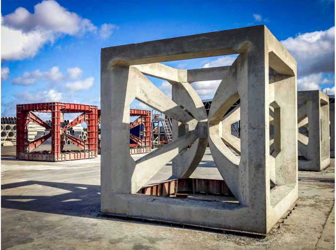
Fig. 2.1: Some of the 60 Fishbox modules being constructed to be deployed in the artificial reefs off Bunbury and Dunsborough. Image courtesy of Haejoo.
