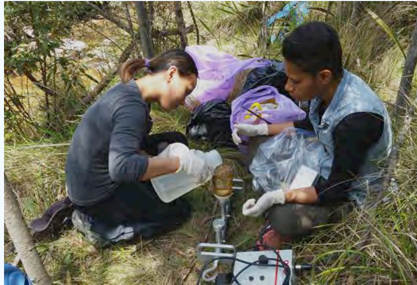
Above In situ pumping of river water to examine for the presence of alien fish eDNA
